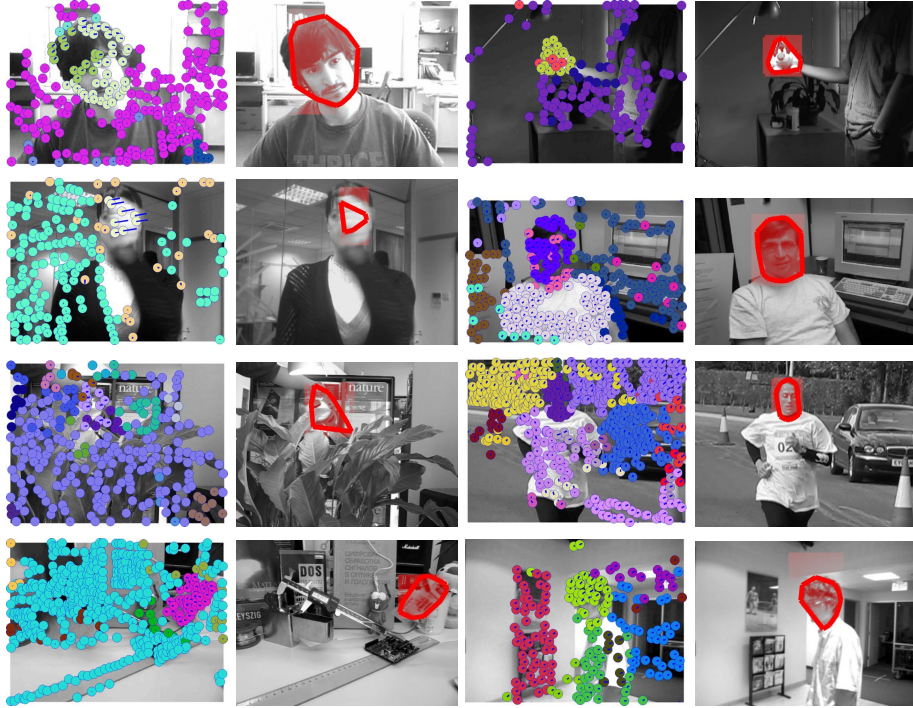
Fig. 4. The Dynamic Objectness groups motion clusters ( 1^{st} and 3^{rd} column; clusters are color coded) into meaningful object regions ( 2^{nd} and 4^{th} column).
