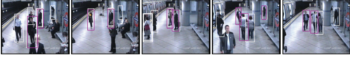
Figure 7. Local detectors (white) trained through information aggregation in specific image regions, compared to the input detector (pink).
