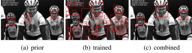
Figure 7. Detection results of a face detector (a) which serves as prior to build a SemiBoost classifier using additional unlabeled data. This classifier alone (b) has not the power of delivering good results but the combination improves the result essentially.
