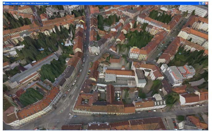
Figure 1: Automatically generated 3D model from a part of Graz. The entire model encompasses 493098 triangles. The image block consists of 155 aerial photographs taken with the UltraCam D camera. Courtesy Microsoft-Virtual Earth, K. Karner.
