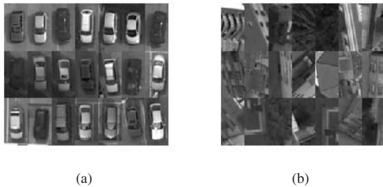
Figure 4. The positive (a) and negative (b) samples used for updating the classifier. The positive samples are hand labeled and given in advance, while the negative samples are generated autonomously.
