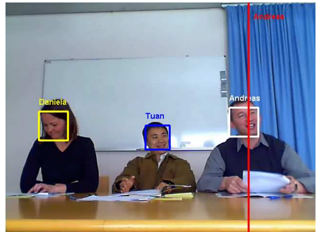
Fig. 3. Visualization of extracted audio (red vertical line) and video information (colored rectangles) at a single timestamp (frame 2175) as suggestion for the user of the annotation tool. Audio and video show the correct result.
