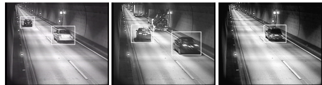
Figure 7. Results obtained by the final car classifier using conservative learning.
